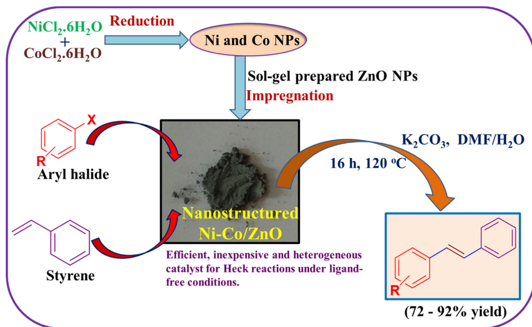
Fig. 1 A detailed scheme depicting the synthesis of nanostructured Ni-Co/ZnO material and its further application in the Heck reaction.
