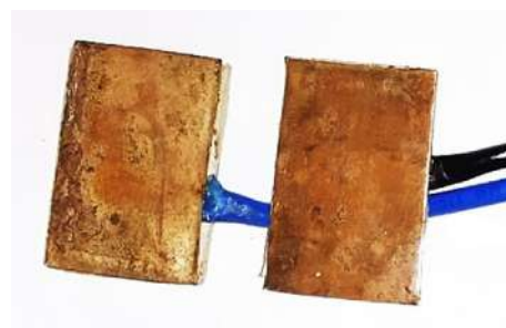
Fig. 1. Photograph of parallel plates of designed capacitor.
