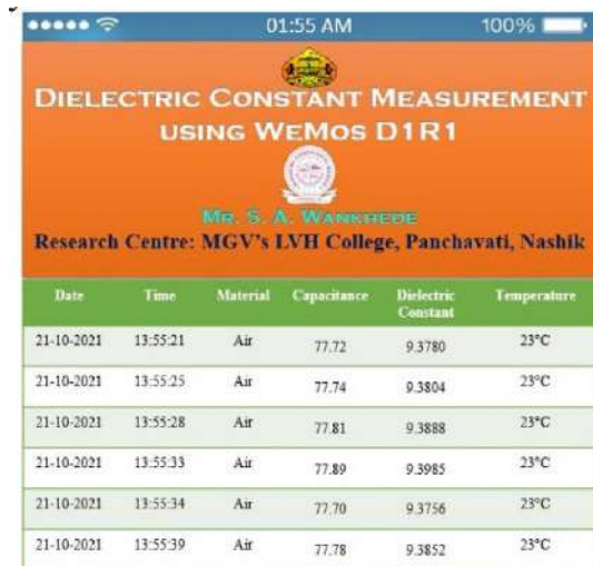
Fig. 5. Screenshot of designed Android app showing readings of dielectric constant measurement system.
