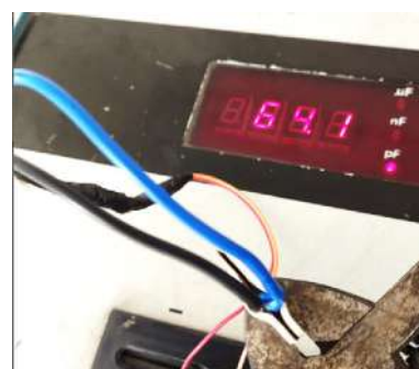
Fig. 2. Photograph of designed capacitor with air as dielectric medium for capacitance measurement using LCR meter.
